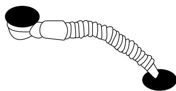
Lift the rear part of bottom basin, and then insert one end of the pipe into the drainage hole
